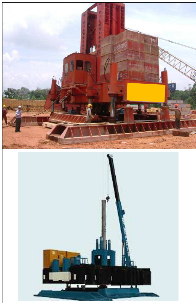
Fig. 17 Typical high capacity jack-in pile machine in Malaysia.
