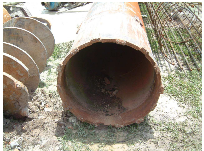
Fig. 13 Modified rock coring tool for bored pile construction in limestone areas.
