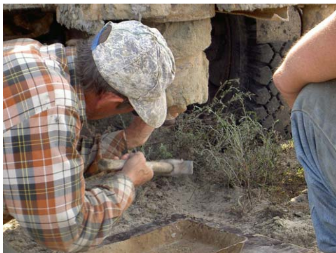
Fig. 28 Collection of disturbed samples from drill auger.
