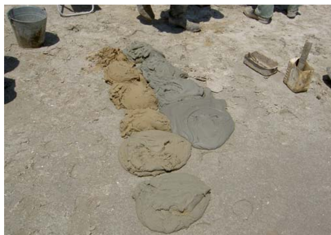
Fig. 26 Drilled materials obtained during SI.
