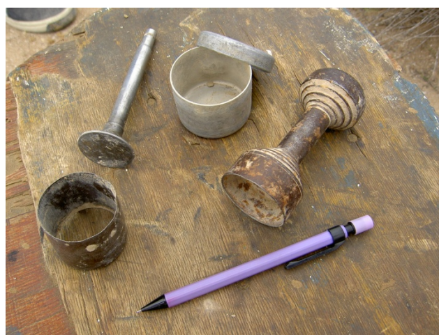
Fig. 27 Apparatus for collection of soil samples.
