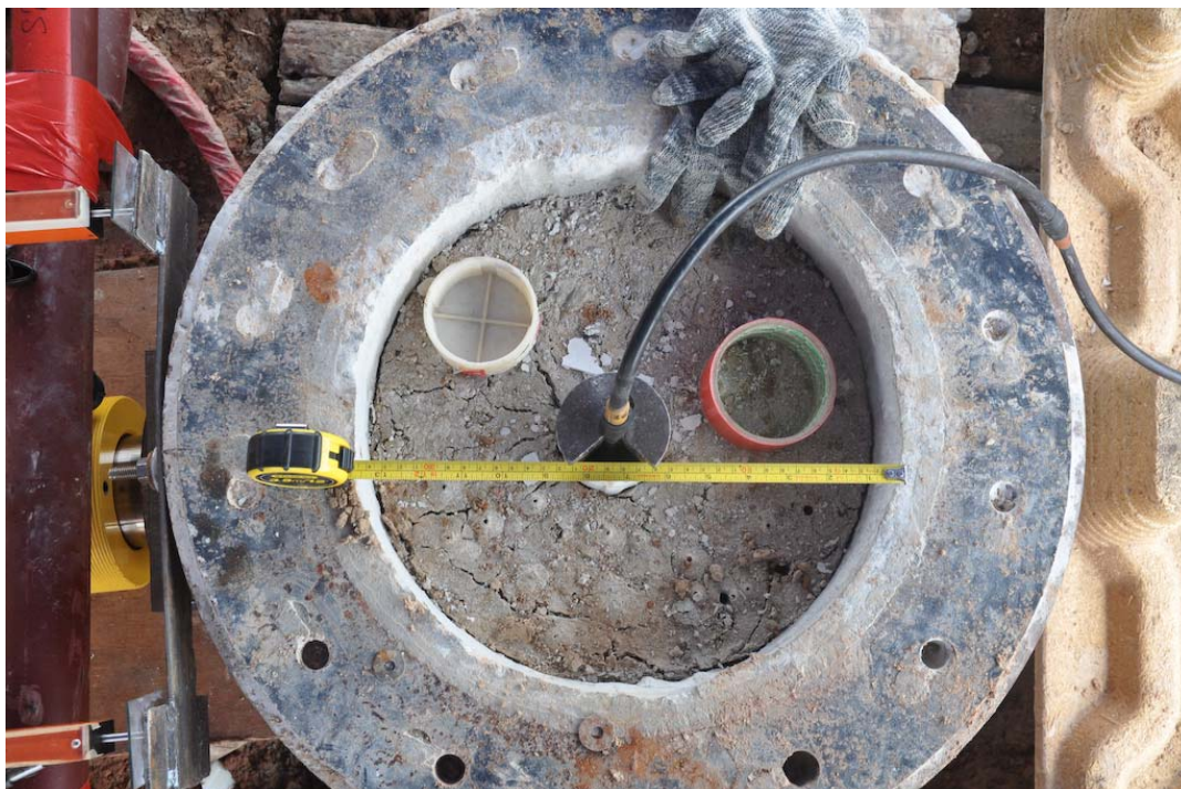
Figure 16: Top View of Test Pile with Inclinometer Tube
